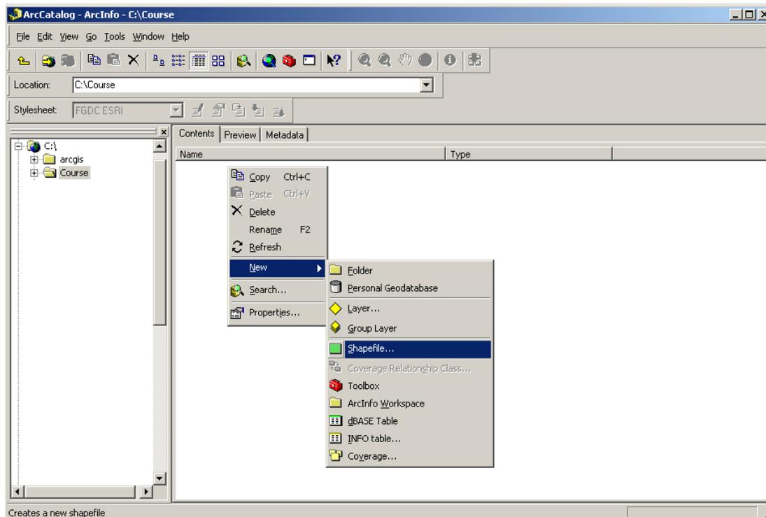
3. In the *Create New Shapefile* Dialog, choose a file name, the type of file (point, line or polygon), and choose a projection by clicking the edit... button. Choose the *Select...* button in the *Spatial Reference Properties* dialog to choose the desired projection from a list. Although ArcMap can “project on the fly” it is important to use the same projection for all map layers in a project in order to preserve accuracy. Click *OK* twice.
